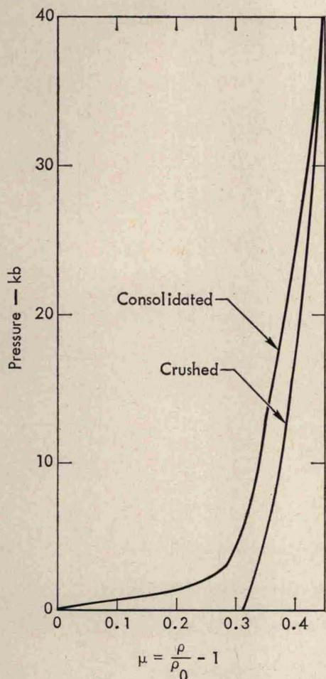
Fig. 11b. Details of lower-pressure portion of consolidated and crushed  $P$ - $\mu$  curves for Marvel alluvium.
